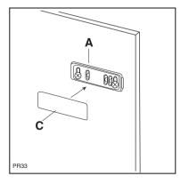
Open the appliance door and the furniture door at  $90^{\circ}$ . Insert the small square (B) into guide (A). Put together the appliance door and the furniture door and mark the holes as indicated in the figure. Remove the squares and drill holes with  $\emptyset$  2 mm at 8 mm from the outer edge of the door. Place the small square on the guide again and fix it with the screws supplied.
